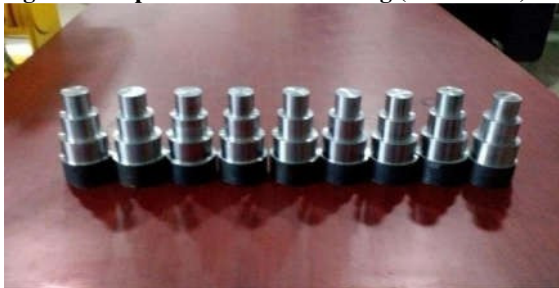
Fig 3. Work pieces after machining (EN19 Steel)
