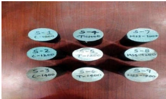
Fig 2. Work pieces before machining (EN19 steel)
