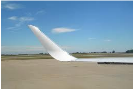
Fig.3: Wings with Winglet
