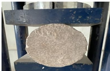
Figure 3. Tensile Strength on Cylindrical Specimen
