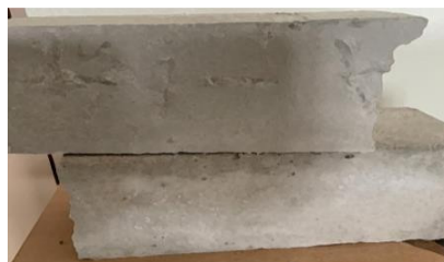
Figure 4. Failed Beam Specimen from UTM
