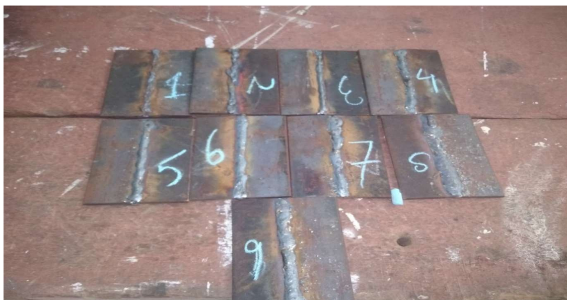
Fig 4. Weldments From The Trails
