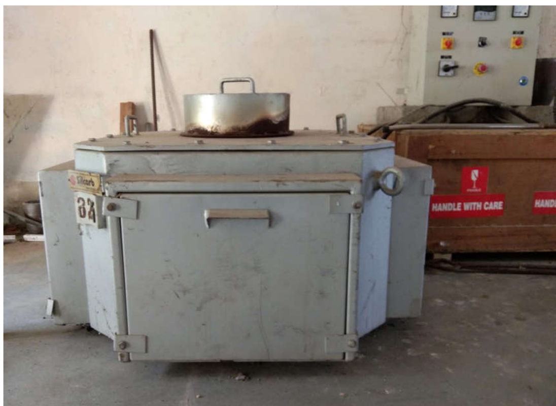
Fig.1 Electric resistance furnace with controll unit.
