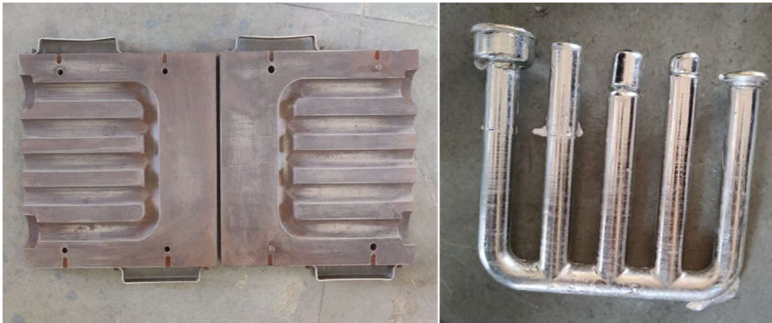
Fig.2 (a) Metallic Die (b) Casting after solidification
