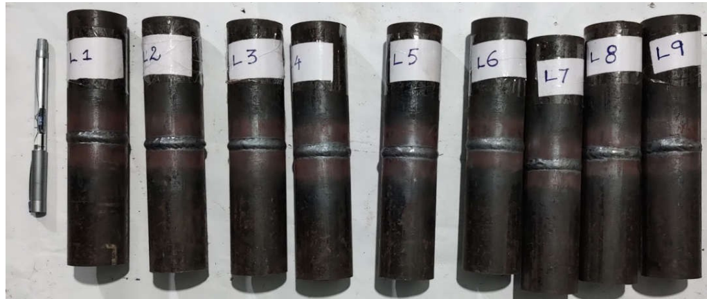
Figure 2. 2.25 Cr 1 Mo steel pipe joints
