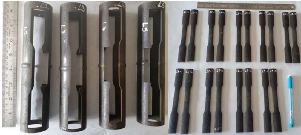
Figure 3. Tensile test specimens
